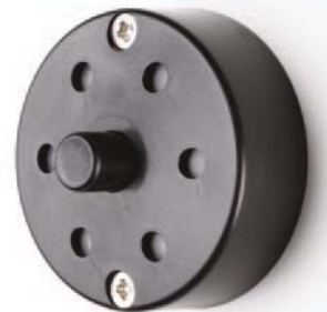
Heated air vent with ice-cleaning plunger prevents vacuum formation, allowing the door to be quickly opened throughout the day
